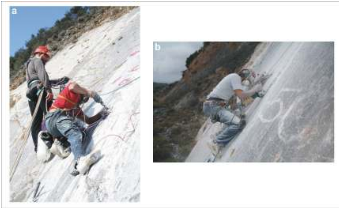
Figure 3: Sampling the lower 15 m of the Spili Fault at Site-1 for REE analysis (a) and the lower 9 m at Site-2 for cosmogenic dating (b) using a portable drill and rock-saw, respectively.
